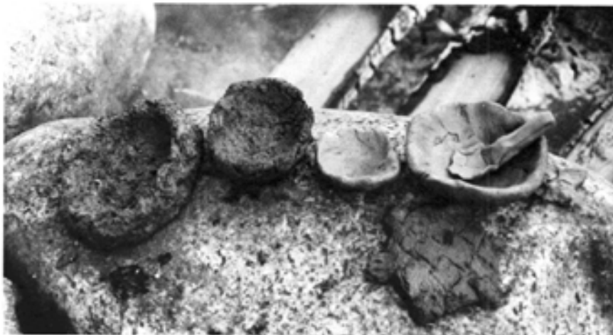
Pottery drying by the fire before firing. Pieces must be thoroughly air-dried before they are fired so that they won't explode as water in the clay expands and turns to steam.
